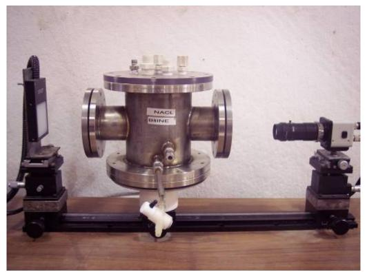
Figure 7: A goniometer with a camera and a light source, used to capture contact angles of oil droplets in a water phase or water droplets in an oil phase (Courtesy of Xuanping Tang).
