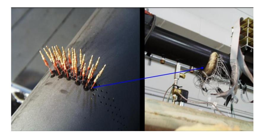
Figure 1. Flush-mounted wall conductance probe for phase wetting determination on the pipe surface
