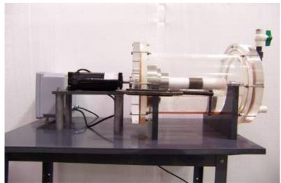
Figure 8: Horizontal rotating cylinder is a benchtop apparatus designed to assess wettability under flowing condition.
