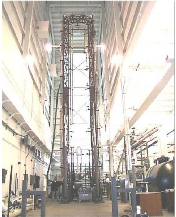
Figure 3. Fully inclinable flow rig at Institute for Corrosion and Multiphase Technology at Ohio University.
