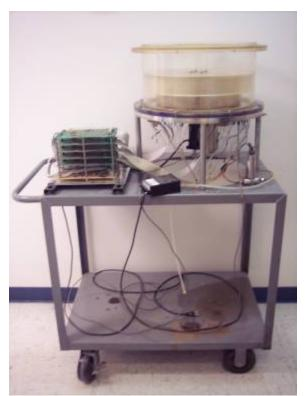
Figure 5. A prototype of a doughnut cell for phase wetting determination (courtesy of Chong Li).
