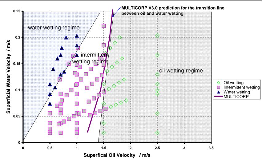
Figure 2. Phase wetting map for LVT200 oil and water two-phase horizontal pipe flow including a line predicted by MULTICORP for a transition between oil and water wetting.
