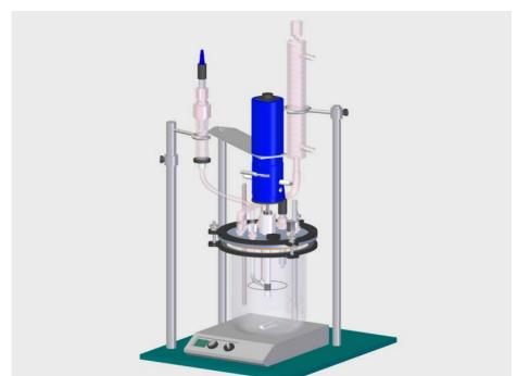
Figure 9: A three electrode glass cell set-up with a heater/stirrer, rotator, lugin capillary, condenser, reference probe, platinum counter electrode and a rotating cylinder working electrode (Courtesy of Haitao Fang).
