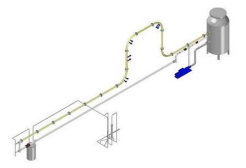
Figure 4: Hilly terrain flow loop is employed in order to investigate wetting in bends (Courtesy of Josh Addis).
