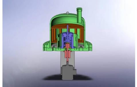
Figure 6: A cross section view of the stainless steel, high temperature, high pressure doughnut cell (Courtesy of Al Schubert).
